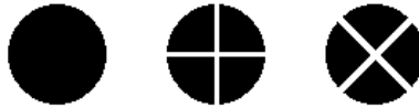
Figure 6.8. Pads are displayed different ways depending on their connection to the Power or Ground planes. From left, a regular pad with no connection, a pad that is connected as a “thermal relief”, and a pad with a direct connection.
