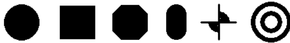
Figure 4.7. Select from several different shapes of pads. From left, Circular, Rectangular, Octagonal, Rounded Rectangle, Cross Hair Target, and Moire Target.
