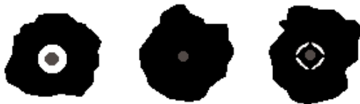
Figure 6.9. This represents how pins actually connect to the solid copper planes when the Board is manufactured. From left, a pin with no connection to a plane, a pin with a direct connection, and a thermal relief connection.
