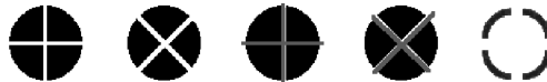
Figure 4.8. From left, a Relief to Power Plane, Direct to Power Plane, Relief to Ground Plane, Direct to Ground Plane, and Thermal Relief pad.
